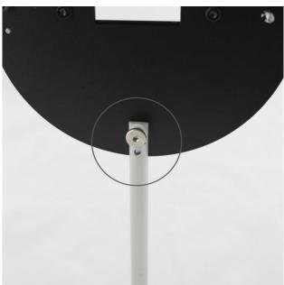
Adjustable rod to change the slit orientation
