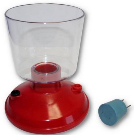
Electrolyser with cap with platinum electrodes
