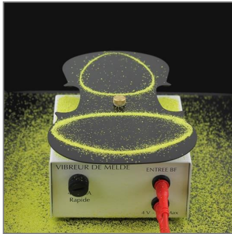
CHLADNI figures on Melde vibrator with violin slab
