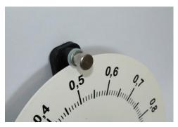
Spiral spring, integrated magnet and knurled screw
