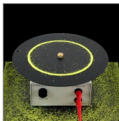
CHLADNI figures on Melde vibrator with the circular slab
