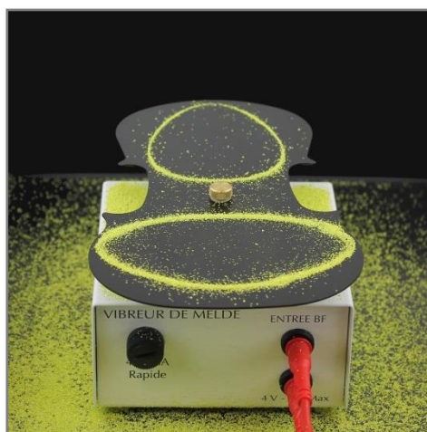
CHLADNI figures on Melde vibrator with the violin slab
