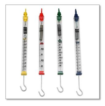
Twinse range of dynamometer peson
