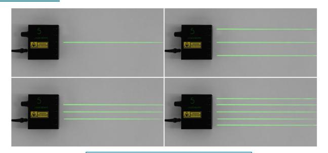
Use on magnetic board with 1, 3 or 5 beams
