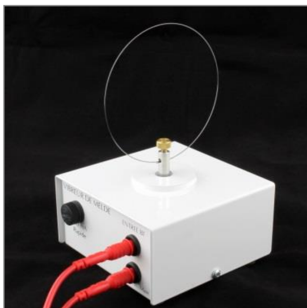
MELDE experiment with circular MELDE rope
