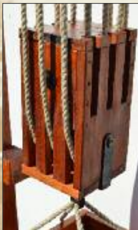
Machines Hellenistic Pulley
