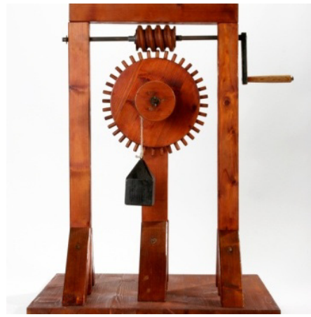
Above: Corkscrew mechanism (Meccanismo Elicoidale) LV 07 Codex Madrid I F.17v
