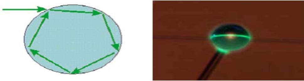
Fig. 1. The total internal reflection of the fluorescence line within the \mu -sphere.
