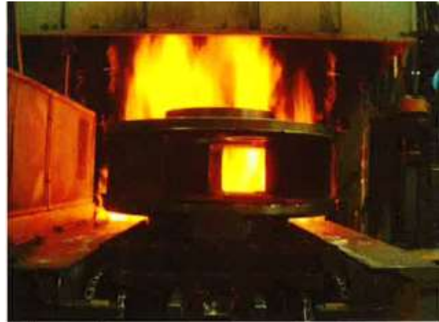
Fig. 22. A photograph of a 7 metric ton ductile iron gear carrier for a wind turbine gearbox being transferred into the vestibule of the furnace as a
